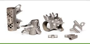
Completed 3D Printed Metal Bicycle Parts
