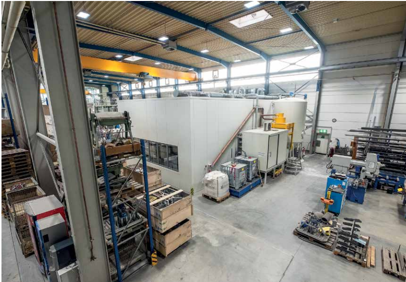
The printing room from behind. There's a refrigerator for chemicals as well as a large sand silo for automatically filling the ExOne 3-D printer.
