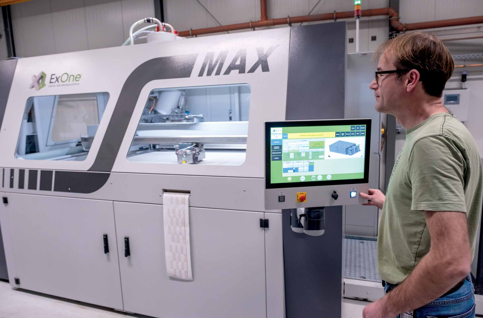
Michael Klein-Hitpass using a 3-D printer. The molds and cores are slotted into the job box like in the classic computer game Tetris
