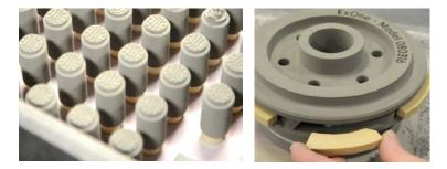
High-density alumina sintering setters printed in 99% purity alumina
