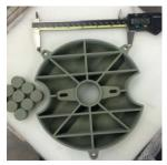
SiC optical structure 3D printed preform
