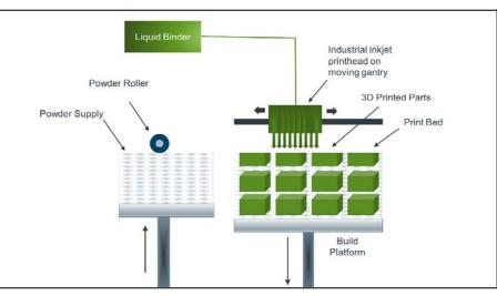
**Definition:** A method of 3D printing in which an inkjet print head quickly deposits a bonding agent onto a thin layer of powdered particles, either metal, sand, ceramics or composites. This process is repeated, layer-by-layer, using a map from a digital design file, until the object is complete.
