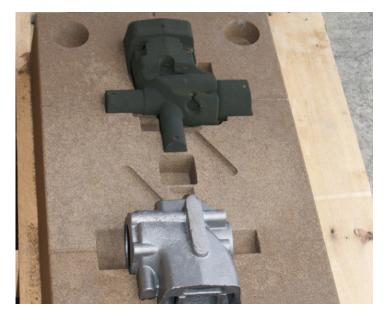
Morel Industries needed a solution to eliminate the human error in the assembly of core boxes used with traditional wood and sand patterns. Working with a local pattern shop with CAD knowledge and expertise, Morel was able to combine 3 cores into 1 printable ExOne core with vents and intricate geometry for their customer. With ExOne's digital printing process, 3 cores were combined into 1, decreasing the scrap rate from 9% to 1%. Lead times were reduced by 60%. Costs were slashed by 85%.
