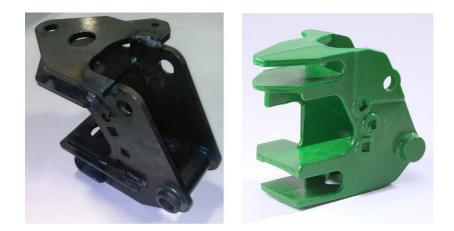
Amerequip required a conversion of their 11-piece, lasercut welded assembly which in turn, would reduce weight, improve quality, and minimize cost through improved production efficiencies with a one-piece design. Amerequip turned to Neenah Foundry, which created the single ductile iron casting design to be made using a single low-cost core. Neenah used 3D printed cores produced at Hoosier Pattern on an ExOne's S-Max system.
