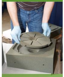
Complex molds and cores in days instead of weeks and months. Pattern-less production for sandcasting.
