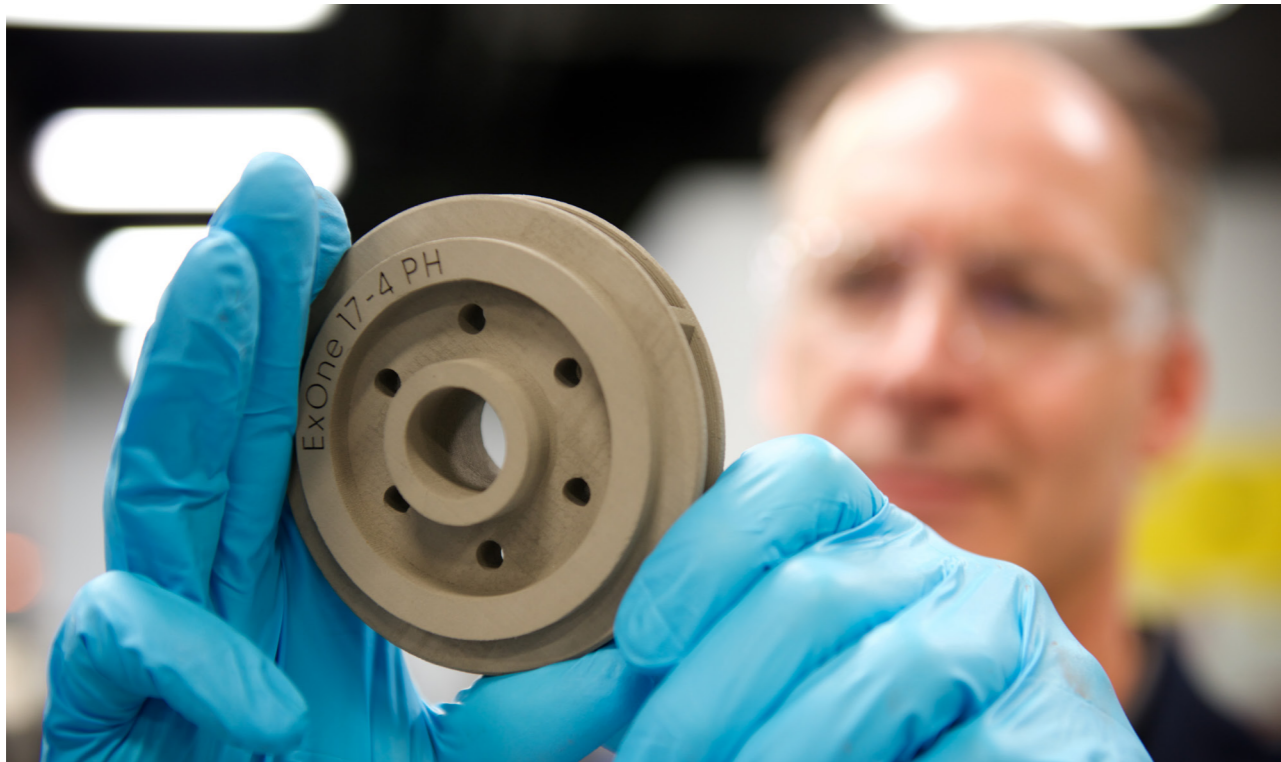
Endless powder: A thin layer of metallic powder material is applied to the construction platform and by a laser or electron beam melted. This process includes selective laser melting and electron beam melting.
