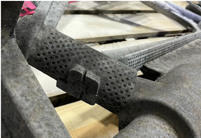
Top left: The 3D printed sand mold from Liberty Pattern is prepped for casting. Top right: The FCS Pascal Process utilized to cast the prototype at Craft Pattern and Mold. Bottom left: The prototype casting ready for post-processing. Bottom right: Next-generation Heavy Bikes are cast at Denison Industries and x-rayed by the foundry to verify the solidity of the aluminum frame.
