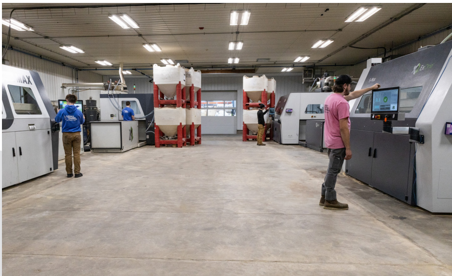
A fleet of five ExOne S-Max sand binder jetting systems at Liberty Pattern in New Liberty, Iowa, allow the company to produce foundry molds and cores with flexibility, even for low-volume projects.
