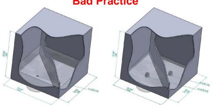
The internal bosses will prevent loose powder from flowing out of the hole
