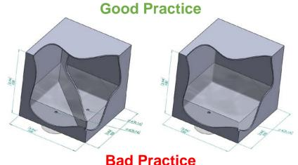
The full cavity has access to a loose powder removal hole
