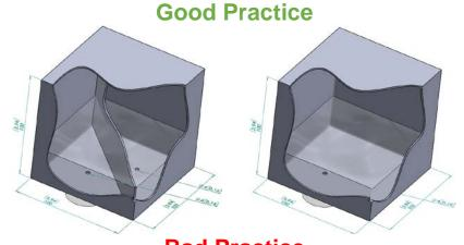
The full cavity has access to a loose powder removal hole
