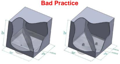
The internal bosses will prevent loose powder from flowing out of the hole
