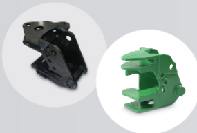
2019 AFS Casting of the Year This casting, enabled with ExOne sand 3D printing, consolidated 11 assembled part into one piece that reduced weight by 2.2 lbs and eliminated traditional tooling.
