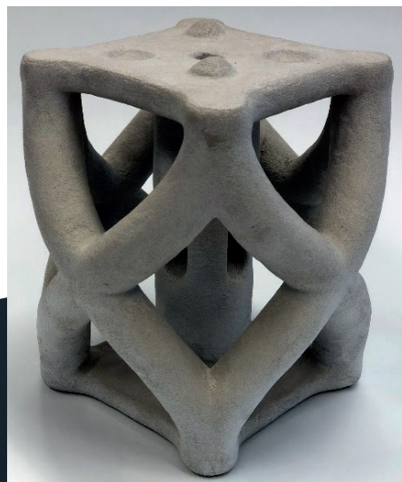
Geometric sample printed in concrete with binder jet 3D printing by Lehigh University.
